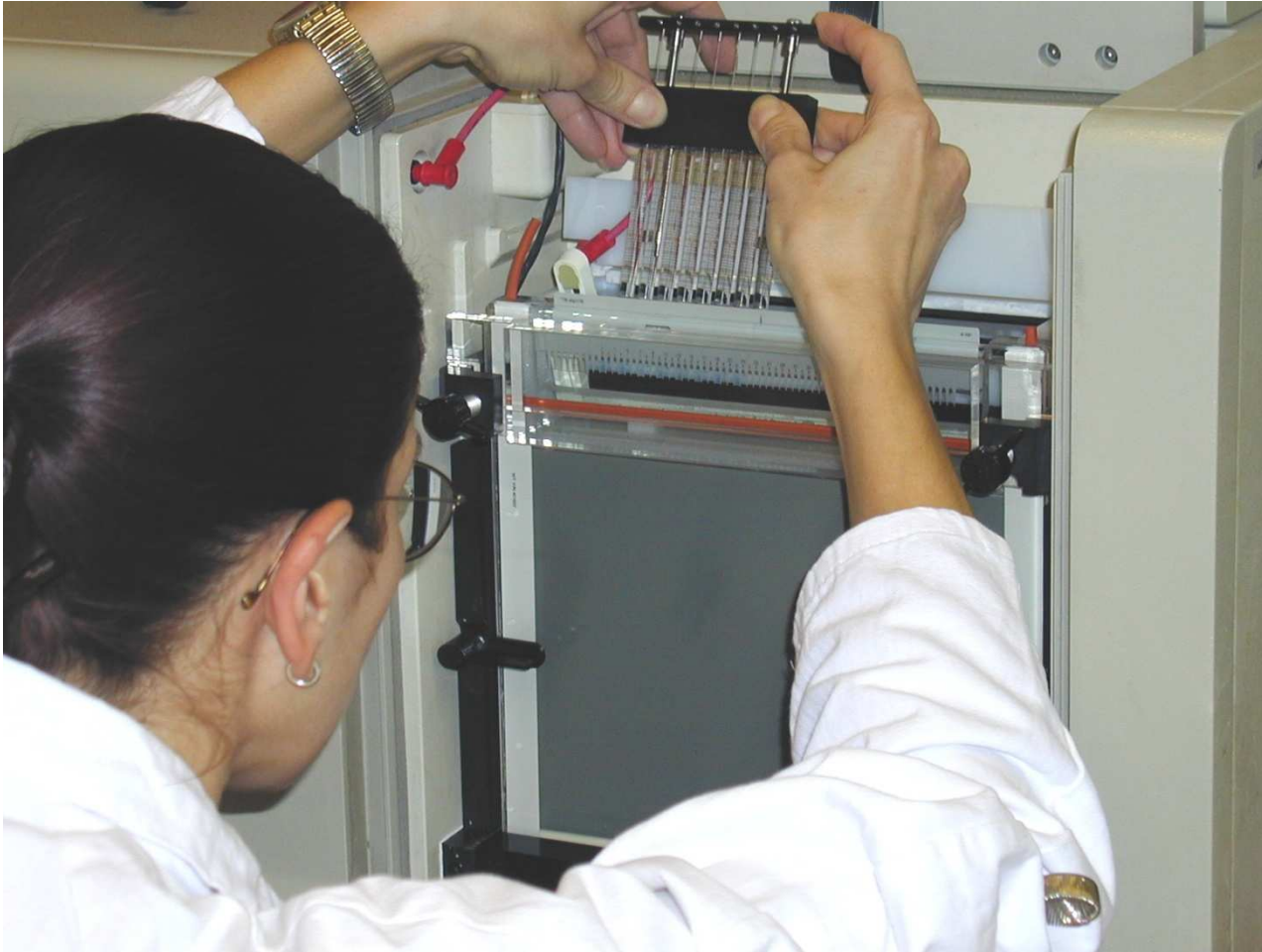
Loading an ABI377 for genotyping
